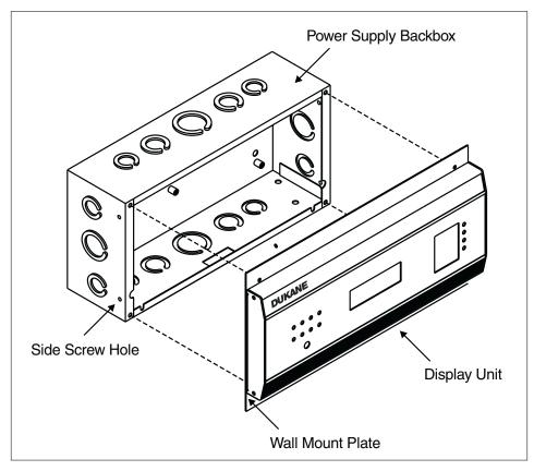
Figure 1-1 Master Clock Wall-Mount Assembly Parts
